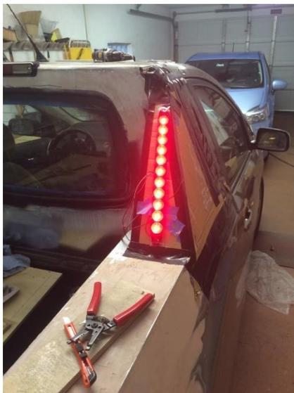
then were incorporated in the fairings and were bright enough to serve as brake lights by themselves. Had I thought this out properly before hand, I could have safely removed all of the brake light section in the original tail lights, giving me more of an area to work with and achieve adequate strength here. I could have also shaped that area so that the rear tail light assemblies could be removed.
