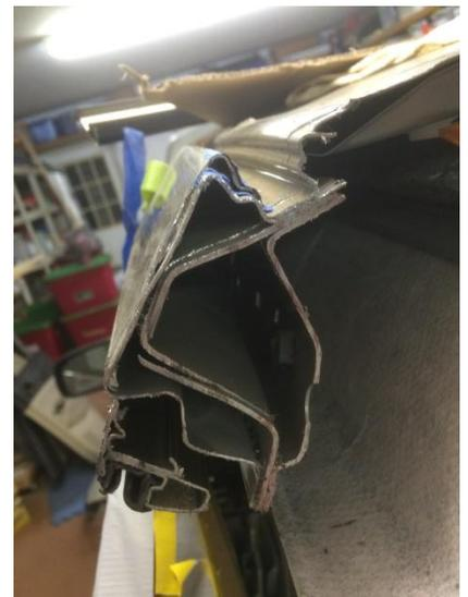
and 2) it would have been difficult to weld this into this junction due to the complex structure of the unibody roof edges (see picture).
